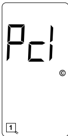
Loop Check Pending Indication
