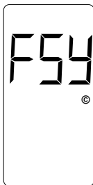
Series Synch Mode Failure Indication
